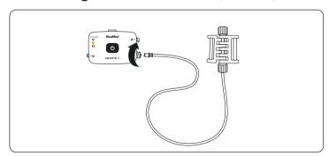
Unscrew and remove the protective cap and insert the connector end of the effort sensor into the effort sensor connector on the device. Turn clockwise until the connector is secure.
