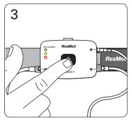
3. Press and hold the power button for about three seconds to turn off the device.
