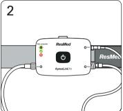
2. Check that the test complete indicator light is lit and green. This means the test is complete. If the test indicator light is red, replace the batteries and repeat the test tomorrow night.
