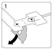
1. Remove the backing from the sensor.
